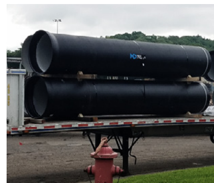
Cement mortar linings, with or without sealcoat, prevent tuberculation regardless of water chemistry.
