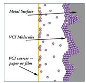
molecules. VCI molecules are attracted to the surface to produce a strong polar bond, hydrogen film, thereby regaining control of the corrosion processes.
